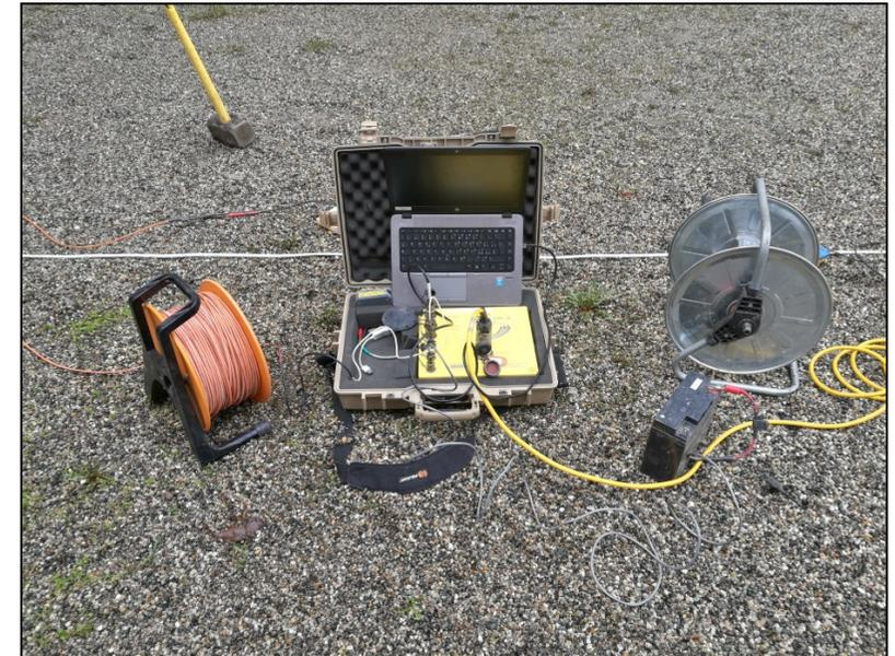
Sismografo Daq Link IV (Seismic Source Ltd.)
